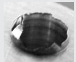
Exit burr with conventional drill
