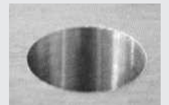
Exit burr with FORCE N drill
