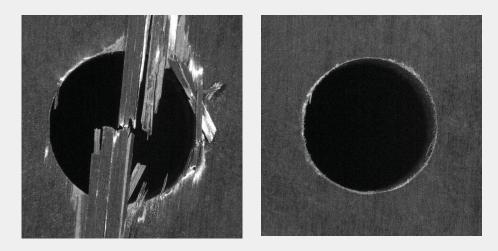
Designed to reduce splintering and delamination when drilling holes in composite materials.
