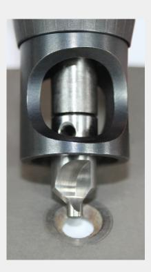
Micro-stop cages used with piloted countersinks helps to ensure a perpendicular approach and enables accurate chamfer depth and diameter.
